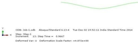
Fig-2: Deflected shape of beam(non-layered approach)
